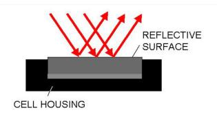
Diagram of Specular Reflectance Standard
