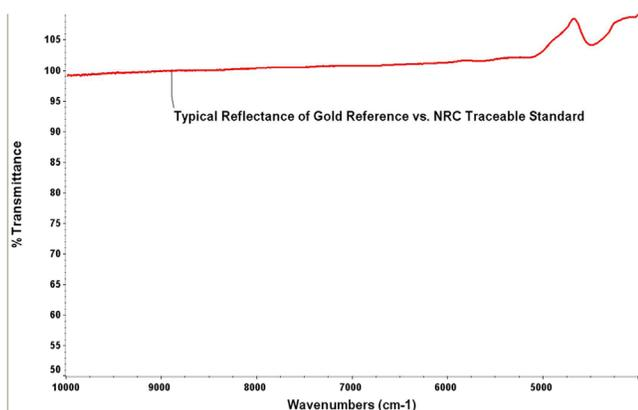
*Measured reflectivity of diffuse gold reference standards is optimal to calibrate other reflectance measurements.*
