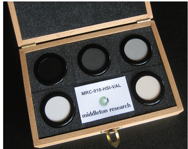
*NIR linearity and wavelength standard kit, including sealed standards of the following nominal reflectance values: white (approximately 99%), 40%, 10%, and dark (under 5%) and a wavelength standard. Standards are delivered in a protective wooden case.*
